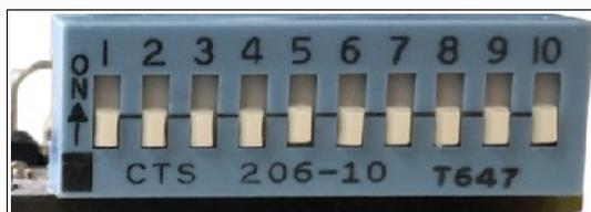
**!!! ATTENTION !!! To decrease the engine cut-off time, it is essential to insert all the selectors progressively from 1 to 10 until reaching the desired "TIME CUT OFF" time portion. If you insert ONLY the chosen one, the device will not work correctly..**
