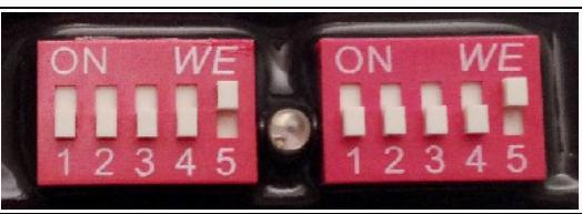
The device is configured by the manufacturer (SP Electronics) during the final testing phase, always on the maximum time of 70 ms which is the recommended starting configuration.
